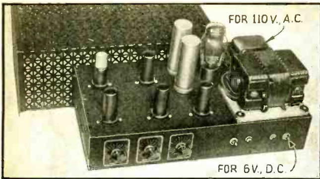
Optional 110 V. A.C. or 6 V. D.C. (arrow should point to genemotor).
