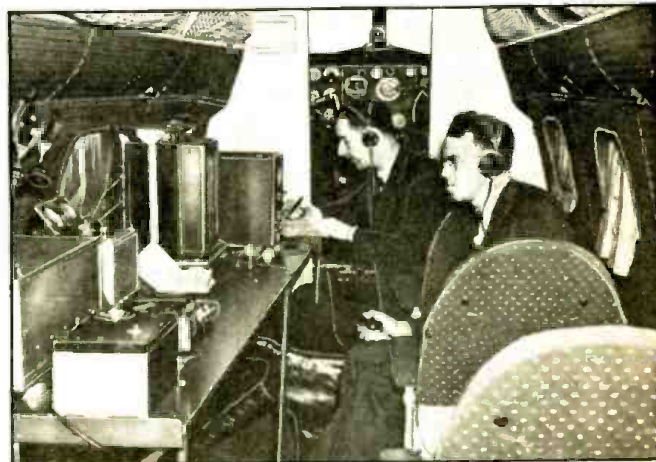
3-MILE-A-MINUTE EXPERIMENTS IN "FLYING LABORATORY" SOLVE AIR-CRAFT-RADIO STATIC MYSTERY. While their flying laboratory speeds along at 3 miles a minute, these United Air Lines technicians (N. E. Klein and H. W. DeWeese, left and right, respectively record their effectiveness of several new types of anti-static aircraft radio antenna developed by company engineers. Upholstered chairs of the big airliner have been replaced by a test stand with delicate recording devices with which the engineers check their success in their battle against rain and snow static which occasionally interferes with plane-ground radio communication. Stripping the mystery from static, engineers aboard the "flying lab." disproved former theories concerning air static and developed the real causes of this communication interference. Company engineers are hopeful that one of the new devices now being tested will solve the problem.
