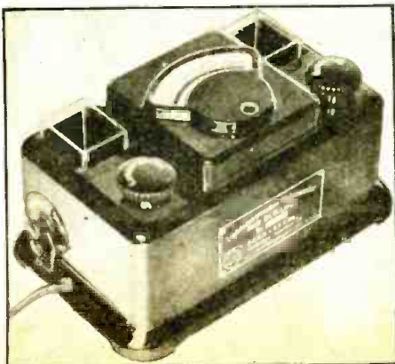
Fig. B. Appearance of photoelectric Colorimeter.
